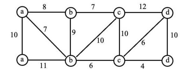
(a) In the tables below, write down the shortest distance from node 'a' to each of the nodes in the graph, when Dijkstra's algorithm is run on the graph.
